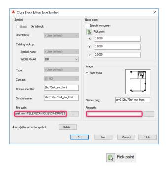
The insertion point of the symbol will be the origin point shown by the X-Y axis.
