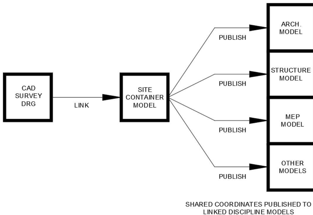
*Fig. Example Schematic of a typical workflow setting coordinates of various discipline's models.*
