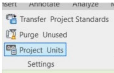
Set the project Unit Length field to 6 decimal places to help with positioning accuracy.
