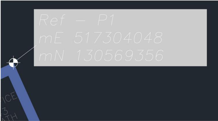
*Fig. Coordinate Reference Point Using attributed fields*
