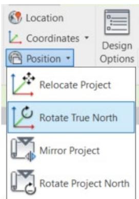
Fig. Rotate True North, is located on the Manage Tab, Project Location panel
