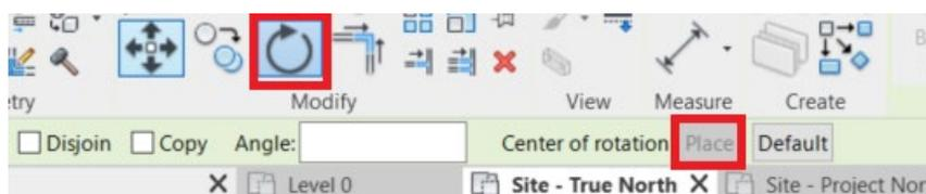
Using the standard Rotation Tool within Revit, rotate the linked CAD file to ensure the major axis of the building or site is Orthogonal to the view.
