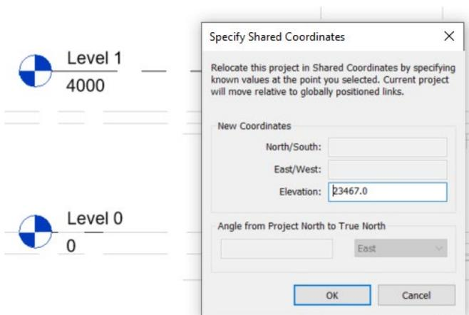
Fig. Specifying level height in container model
