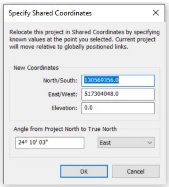
When specifying the coordinates, ensure the correct point is selected and enter the coordinates as shown on the CAD drawing. Revit tends to think in millimetres whilst surveyors tend to think in metres, but provided units are specified correctly in format and units, the coordinate tag should have the same value as the equivalent AutoCAD text.
