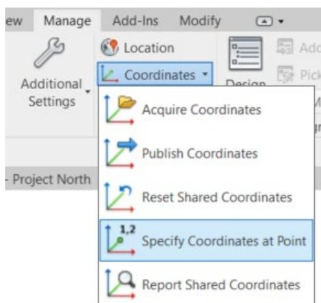
As a check a Coordinate Tag can be placed at the same point. Initially the values will not match, but once the coordination task has been achieved the tag value will be the same as the coordinate text within the AutoCAD drawing.
