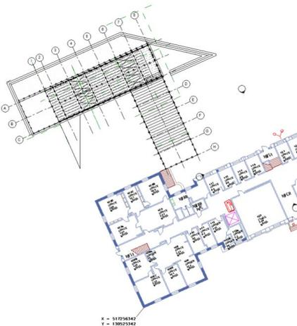
*Fig. Lining up the building model to reference lines*
