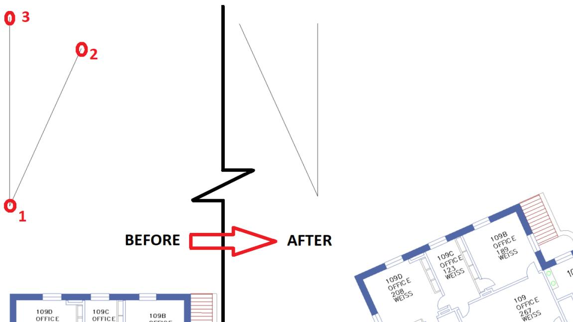
Once complete you should be able to toggle between Project North and True North settings (or view) and see the building orientate to the correct aspect.
