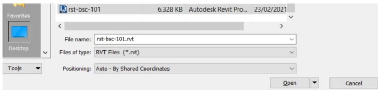
*Fig. Once a Shared Coordinate System has been established, any related files can be linked together and appear in the correct place with this positioning option.*
