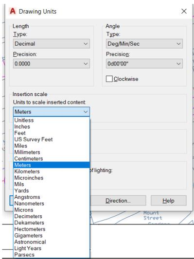
Fig. AutoCAD units should reflect the actual units the file has been drawn in!
