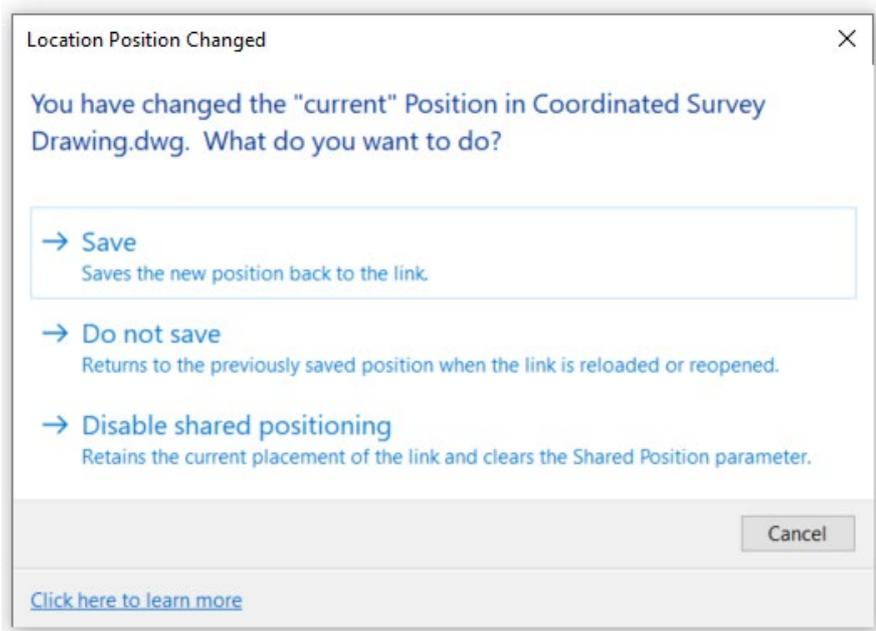
A link has now been established with the linked AutoCAD drawing. The coordinates between the Revit and AutoCAD file should correlate.
