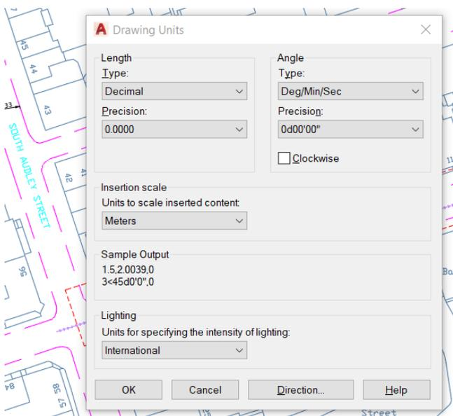
Fig. Survey drawings are typically drawn in metres.
