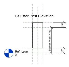
7. Create the column base with a second extrusion. Use the pick draw tool and offset the sketch lines 25mm outside of the width and depth ref planes. Dimension and lock this 25mm offset then finish the extrusion. In the left elevation, align and lock the bottom of the extrusion to the Ref Level and the top to the base height ref plane (150mm above the Ref Level).
