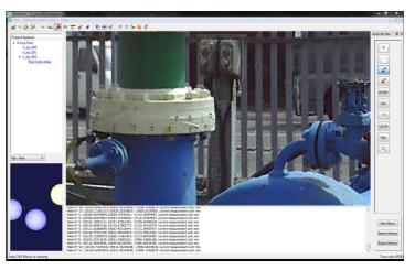
We will use VirtuSurv to help us here as this provides much greater visible acuity. We click several points around the edge of the flange and then further points to locate the flange face. We will represent the nozzle with a flange to aid visualisation, and write the co-ordinates and orientation of the nozzle to the drawing.
