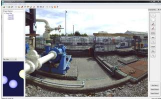
The image above left shows a section of a pointcloud that has been loaded into a drawing in AutoCAD Plant 3D with the kubit PointSense Plant plugin installed. Using the sectioning tools in PointSense Plant, we have clipped out a section of the pointcloud that contains a pump set that is of interest.
