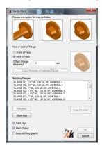
If we start with the flange on the intake of the pump, we have a view of the back of the flange and the straight length of pipe running into it, clearly visible in the pointcloud. So, we choose the Back of Face option in the *Tie-In-Point* window and then click on the method by which we we will define the direction of the axis of the flange – we will do this by clicking two points on the pipe in the pointcloud.
