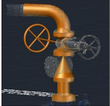
and from the kubit model export an as-built Plant 3D model of the existing lines.
