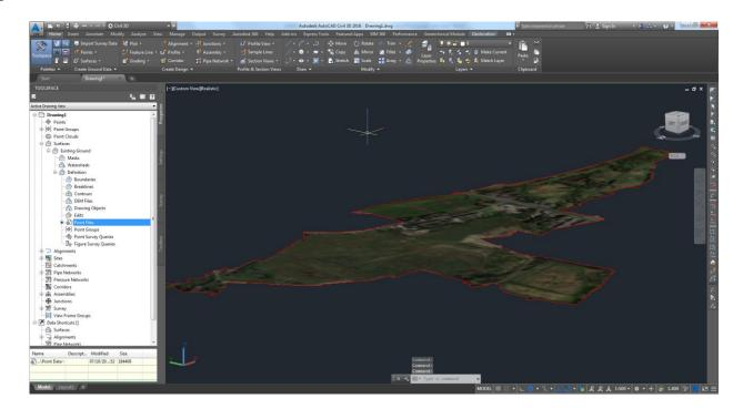
7. This view can be further enhanced by changing the surface display style to a 3D Exaggerated one, this accentuates the slopes and mounds allowing us to view them more easily in a larger context as shown in Fig. 6.
