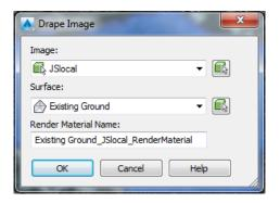
6. Before entering a Realistic 3D view I will unload the aerial photograph so that it does not impede my view. As can be seen in Fig. 5 some impressive results have been achieved and the model looks much more realistic. The image has been bent around my triangulation allowing me a rough idea of current land use and condition.
