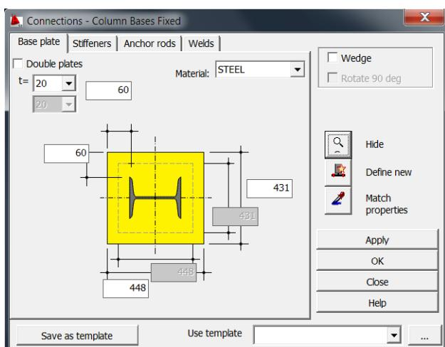
I filled each tab working from right to left to create the base plate dimensions. The dimensions don't have to right first time just selecting the connection again after allows you to open and modify the dimensions as needed.
