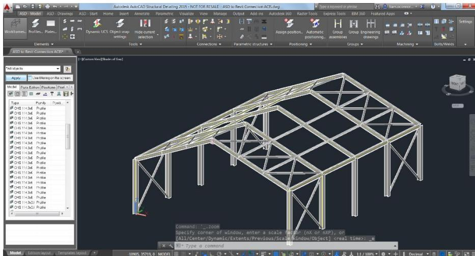
Open an ASD file, I have already created some model geometry already, in this example I used the link from Revit 2015 to Autodesk Robot Structural analysis 2015 (RSA) and then opened RSA file directly from ASD via the drop below the Tools panel. You can create the model geometry directly using ASD also.
