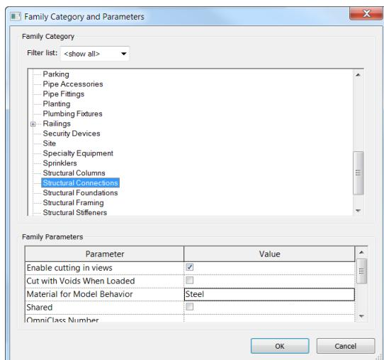
and parameters icon and change the template to “Structural Connections”.
