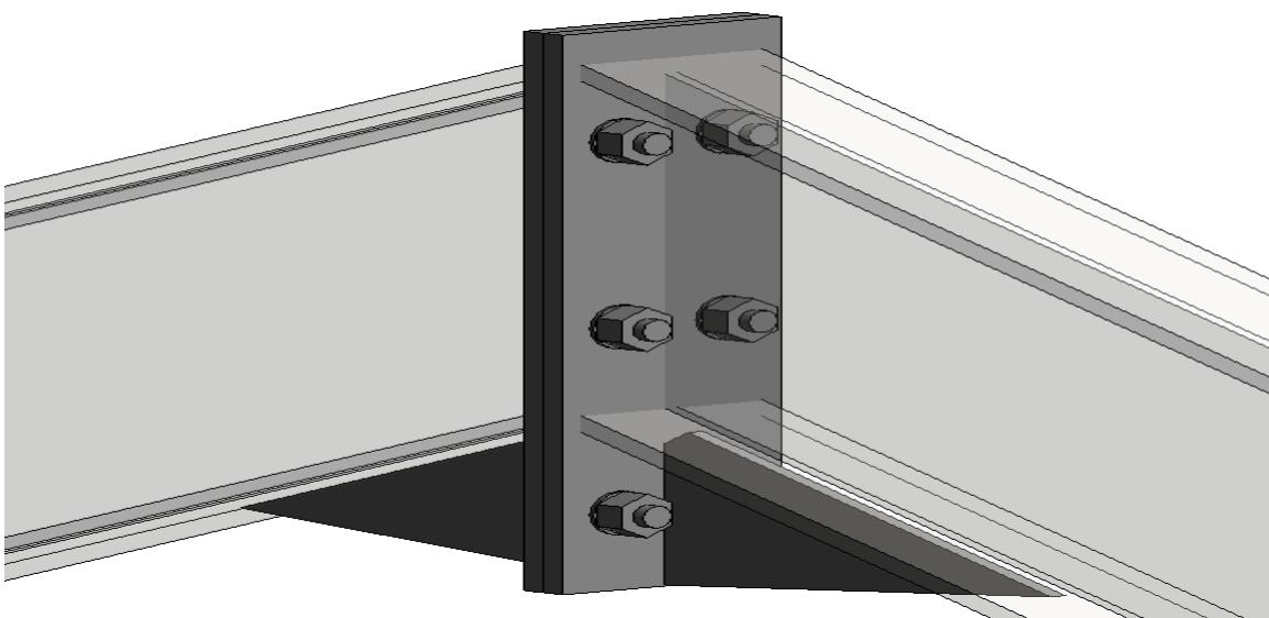
Using the Connection Macro dialog box wizards used in ASD you can produce the varies connection details in 3D ready to produce the 3D/2D fabrication drawings. Using the option to save as “.ACIS” in ASD you can export the connections out and load them in to Revit Family template (shown above).
