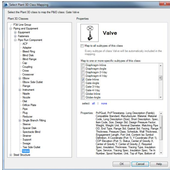
Note that there is only one Valve class in the Plant 3D class list and that it is not possible to extend the list.
