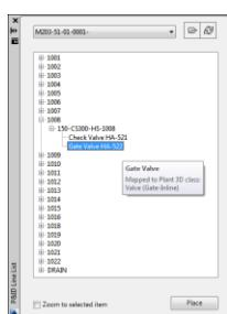
By picking an item from the list and choosing the Place button, Plant 3D chooses a corresponding component of the given size from the defined Pipe Spec ready for insertion into the 3D model. The size and spec are determined from the size and spec of the process line – 150mm, CS300 in the above example.
