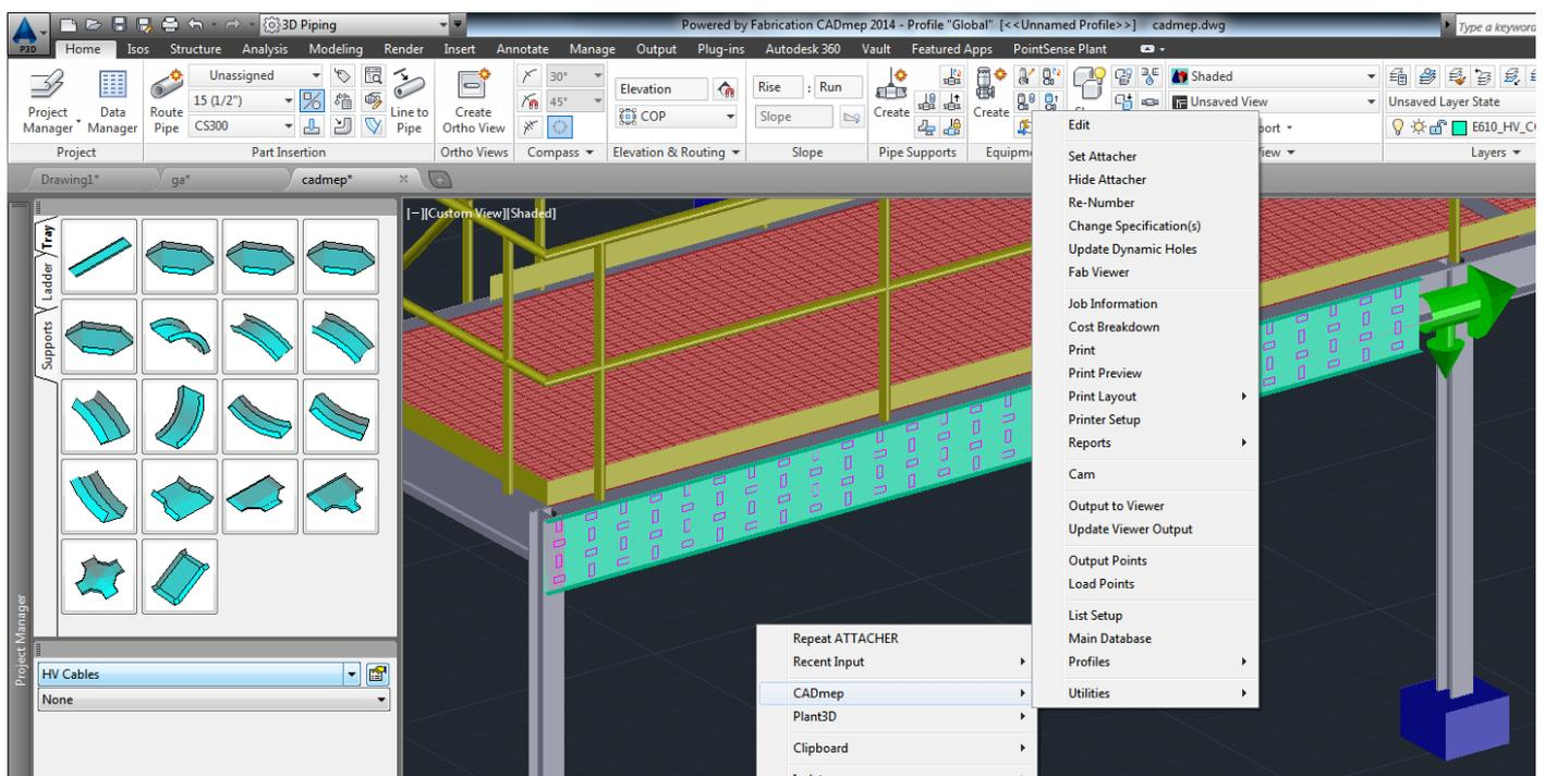
In the example above, a structural drawing has been Xref'ed in to a new Plant drawing and a length of cable tray has been added. If this drawing was now included in an Ortho view, the generated view would be blank.
