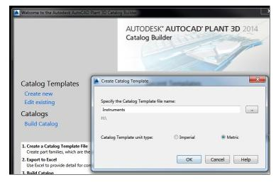
The Part Family list on the left of the Catalog Builder window does not contain an entry for instruments. Because of this, a new Valve family is being created through which the geometry for the new instrument family will be defined.
