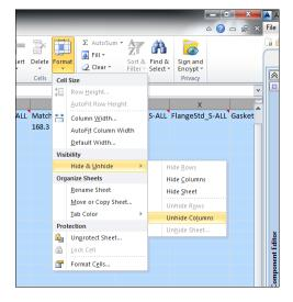
This provides access to the PartCategory and PnPClassName columns which are used to define the family to which the part belongs. These values can now be updated. The PartCategory must be set to Instrument, and the PnPClassName must be set to either Instrument or InlineInstrument depending upon the type of instrument family that is required. In this example, an InlineInstrument is being created.
