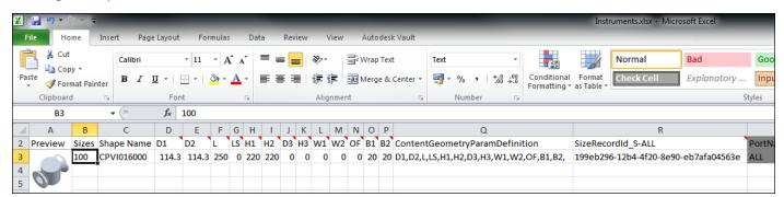
Note that if Block based geometry is selected, then filename and block name columns are included in the spreadsheet rather than size parameters.
