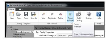
The Excel spreadsheet provides access to all of the data that will be used during catalog creation, including the size parameters for the geometry.
