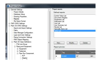
4. The Modify Report windows is displayed. In the 'Report properties' panel, expand Plant 3D Object Properties, expand Valve and tick Model Number.
