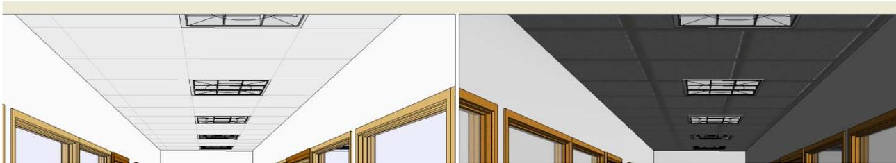
As you can see, in the image above, the ceiling lights align as expected with the surface pattern of the ceiling when it's in a Hidden line visual style; however, once the image had been rendered the materials were out by approximately half a tile!
