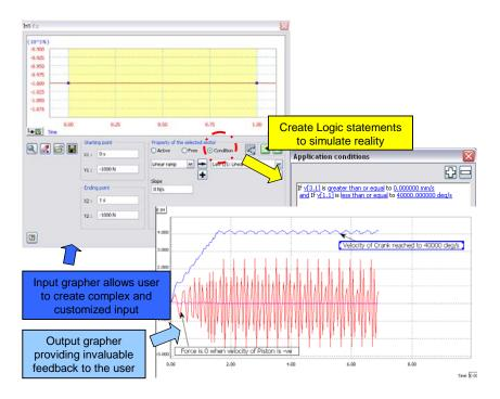
After entering the correct environmental constraints and joints, the designer runs the simulation and analyzes the results using the Output Grapher, as shown in the following graphic. In addition to displaying standard parameters, the designer can also create custom parameters in order to effectively analyze the simulation.
