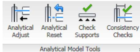
These checks are available in the structural settings – as shown in Fig 12 – as well as directly in the user interface ribbon, under the analytical model tools.
