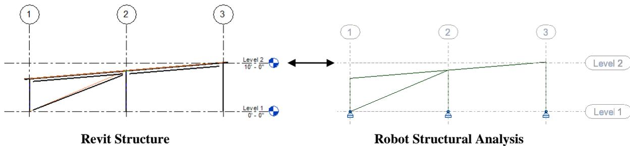
Coplanar framing of a sloped floor having the projection parameter(s) set to “Auto-detect” will automatically align the analytical framing line to the analytical plane of the floor where the floor is set to Top of Slab or Bottom of Slab.
