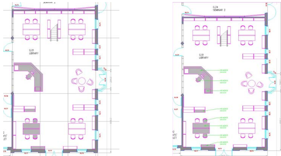
Before and after. This part of the exercise involved annotation of the furniture using common AutoCAD tools
