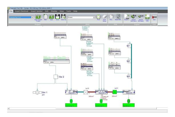
To modify the system simply click on the item to alter and enter the revised values. Recalculation is instant, with cable sizes and other results displayed either directly on the layout or in easy to read schedules.
