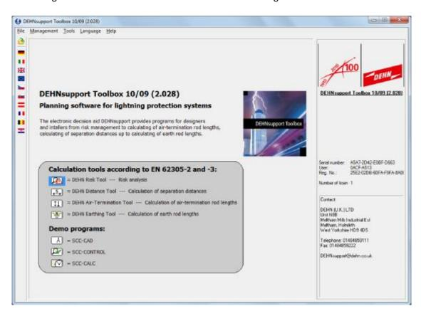
The full risk depending on strike source, whether direct or local with EMP, can be taken into consideration along with all methods of surge protection and fire risk analysis. Separate lightning protection zones can be set up depending on the protection class I-IV which then looks at the "rolling sphere" method of determining protection of obstacles with separate finials.
