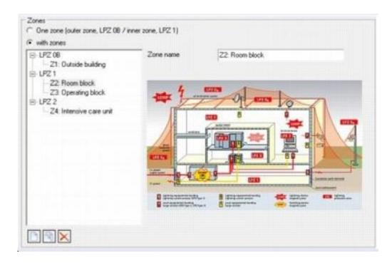
Full separation distance calculations can be used based on the class of lightning protection required, giving minimum separation distances of the earthing system to prevent flashover into internal services within the building.
