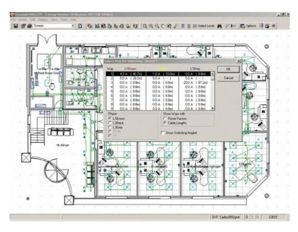
The board schedules developed can be imported into the Cymap Wiring package so cable takeoffs and loadings from the floor plan will automatically populate the schematic.
