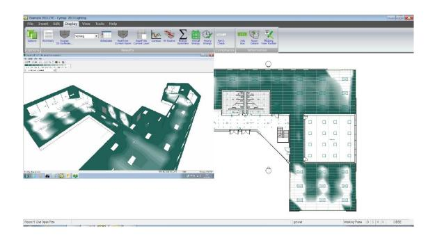
3D rendered images can be created in real time to look at individual rooms or entire floor plans in a 3D format. This allows analysis of lighting on vertical surfaces where feature lighting is employed.
