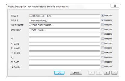
Fill in the revision data in the relevant fields. In this example, we can fill in the R1\* fields as it is the FIRST ISSUE
