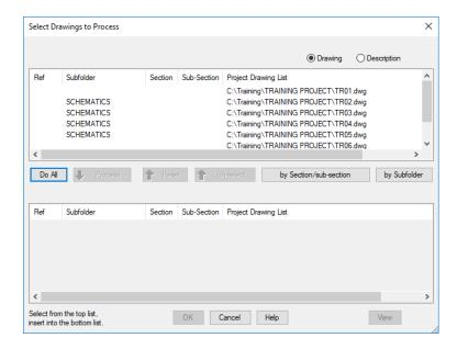
Using *Shift* and *Ctrl* to select drawings, you can decide which drawings to Process. This is extremely useful if you only want up issue an individual drawing or indeed selected drawings rather than the entire project. You can also up-issue the contents of a by Subfolder sub-folder or selected sub-folders rather than the entire project as well.
