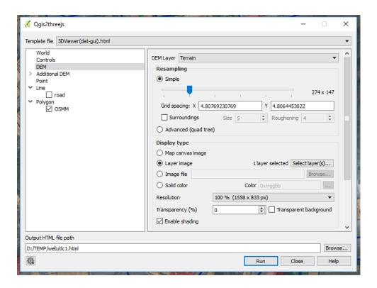
**POINT, LINE, POLYGON** – Depending on the layers you have open in QGIS, you can tick to choose which layers to display, define a colour style, decide to show/hide labels and choose how the layers are extruded within the 3D map.
