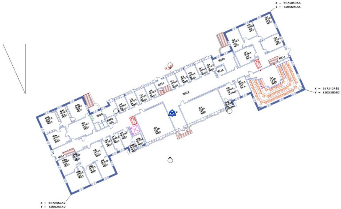
Once imported, Revit needs to be told the Project North, True North Deviation. As AutoCAD defaults to True North by default, but Revit thinks in terms of Project North, the user needs to rotate Revit's True North to the correct direction.
