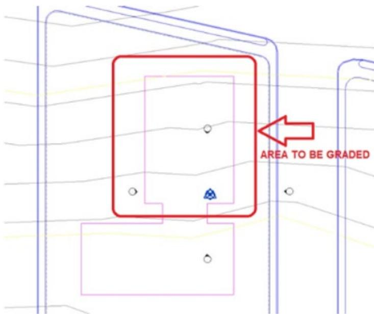
The marked area needs to be flattened. Note the contours crossing over the area to be a foundation or floor slab. The solid can be graded to create a flat area to build upon and can be scheduled to see how much material needs to be removed or added to site. This information will be calculated and accessed via Cut and Fill parameters.
