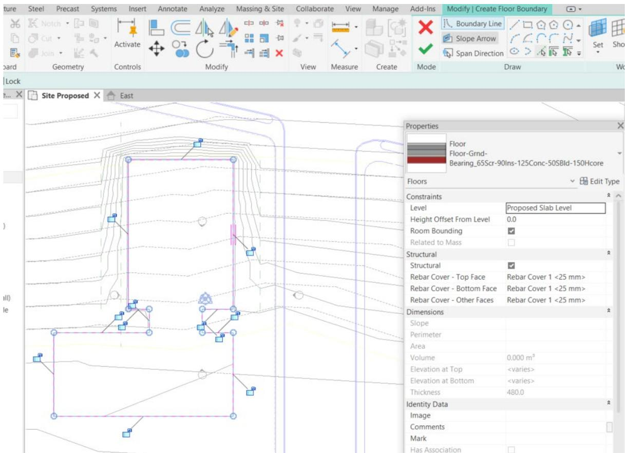
NB. Revit will report that the slab and toposolid overlap. To ensure clean section display and accurate reporting, the slab will need to be cut from or joined with the toposolid. If using the Join tool, select the toposolid FIRST, then the slab to ensure accurate reporting of cut and fill volumes.
