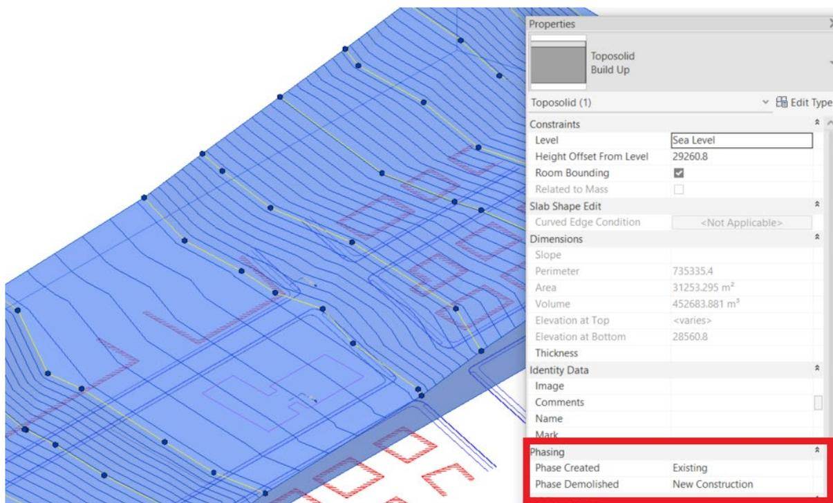
Once complete, switch to a 'new construction' site view. The existing surface should appear grey due to the phase filter applied to that view. Locate the Graded Surface tool to modify the existing site and create a flattened area to add a suitable slab entity.
