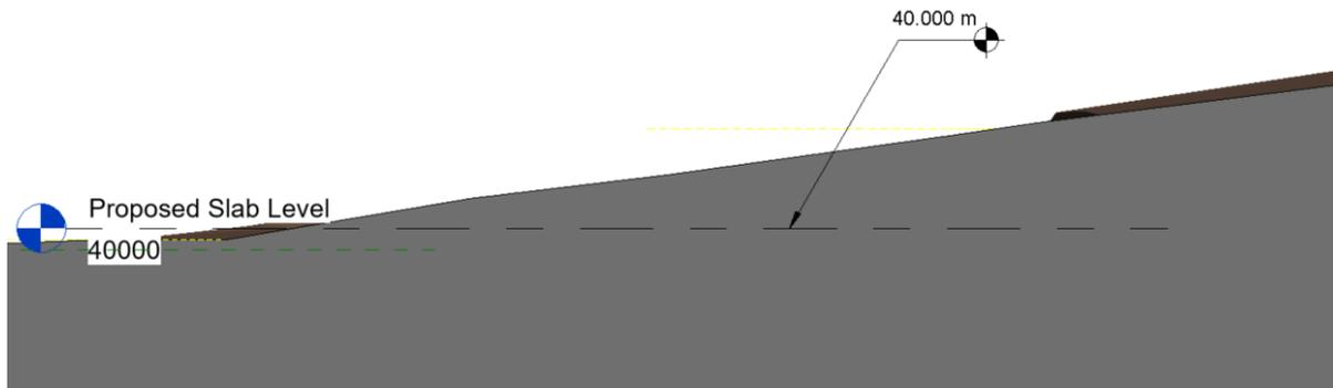
Fig 3. Determining the level for the building slab.
