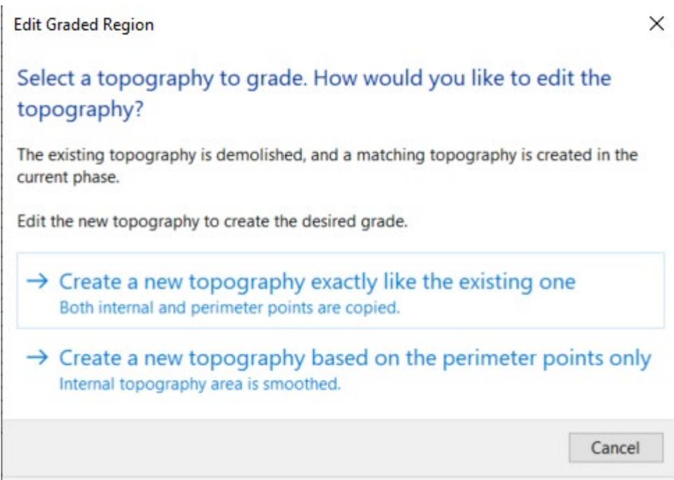
Choose the first option 'exactly like the existing one'. This will ensure better surface modelling accuracy. Use the perimeter points option only on simple flat solids. This will create a new surface which can be adjusted to suit design intent. Most situations will usually require the former option.
