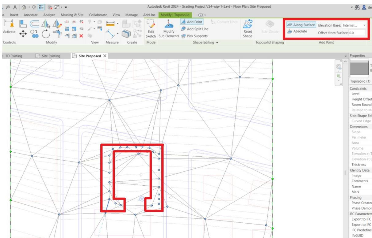
Fig 2. Creating 'top of bank' spot heights relative to surface.
