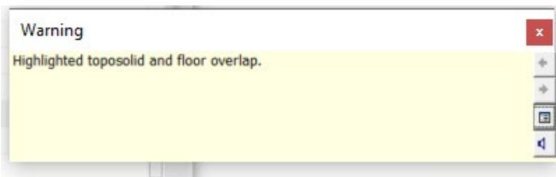
Should there be a need to fill ground to accommodate a slab and other features model a Massing Solid Form. Adjust to suit. This can also be joined to the toposolid which will adjust the cut and fill amounts accordingly.
