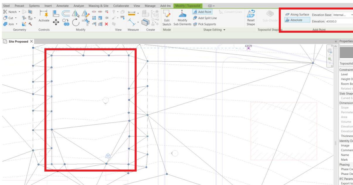
Fig 4. Creating 'bottom of bank' spot heights at an explicit elevation.
