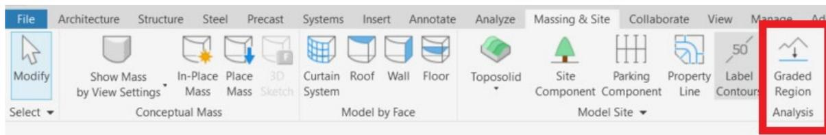
Revit's site tools lack such features like break lines so to control the shape of the toposolid, additional spot heights need to be added to define the bottom and top edges of banking. This will be achieved with the grading tool. Clicking the existing solid to grade will display the following message:
